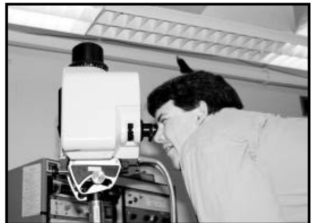
Scott Stevens of Pratt & Whitney West Palm Beach sets up a SPATE scan.
