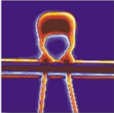
Stress Image of Capacitor
