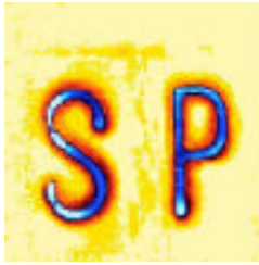
Figure 1. Contact stresses in embossed plastic letters.
