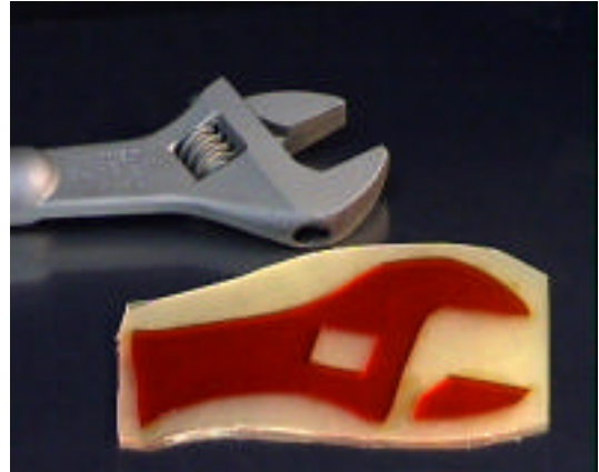
Fig. 5 Allow coating to partially cure
